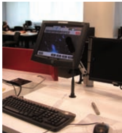
UQ TECHNOLOGY INTERFACE THE TEACHER'S LECTERN PROVIDES TOUCH SCREEN CONTROLS FOR AUDIOVISUAL FACILITIES IN A RANGE OF PRESET MODES.
